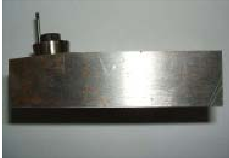
Figure 5. Device for orientation, fixing and dividing for T channels, lateral view.
